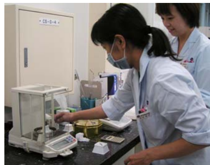
A&D GR series analytical balance and sample cup holder. Compact design with innovative retractable breeze break.
